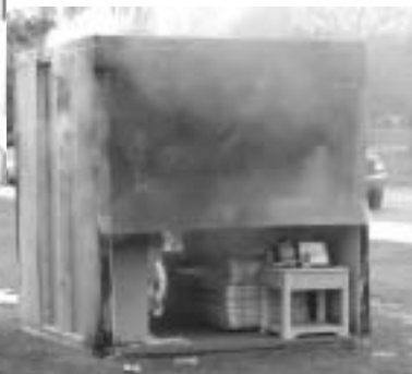
ABOVE - At the Oak Forest demonstration, flashover occurred in the unsprinklered room at approximately two minutes.
